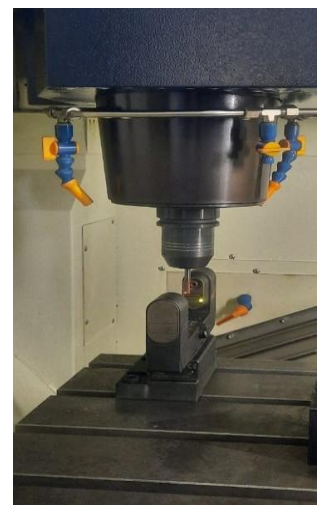
Figure 5: High-precision probing of a compact
