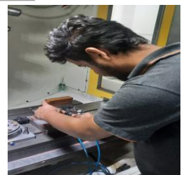
Figure 6: Operator performing job setup on VMC
